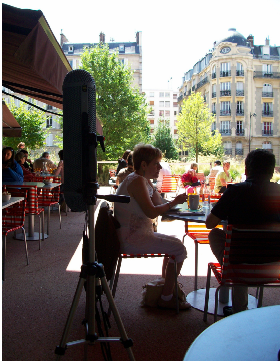
Figure 3—5 Café noise recording, showing microphone wind-shield on tripod
